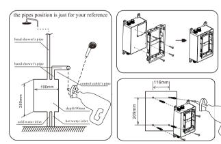
Step 4 Connect the water pipe and the power supply cable of the host box, get water supply to test the pipe no leak. Lead the host box control cable out to the control panel's bracket and temporary fasten it. And then use the cement to seal the wall and cover by the tiles.
