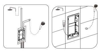
Step 5 Connect the control cable between the host box and the control panel, putting some silicon on the back case of the control panel and put it on the wall bracket.
