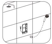
Step 6 Connect the control cable between the host box and the control panel, putting some silicon on the back case of the control panel and put it on the wall bracket.
