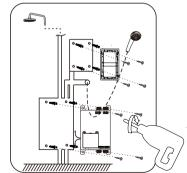
Step 4 Install the wall bracket of control panel and the host box in two holes, according to the pipe's position to set the host box position, adjust the screw of wall bracket to make sure it is concave the wall surface with 0.5-1 mm difference.
